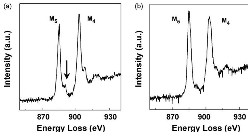
**Fig. 4.** (a) EEL spectra of Ce-M edge at zero bias. (b) A reversal in the intensity of Ce  $M_{45}$  white lines was observed; and the shoulder indicated by arrow in (a) disappeared after applying the electric field.
